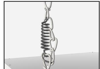
**1** Place fastening hooks on the strapping board or the floor joists.
