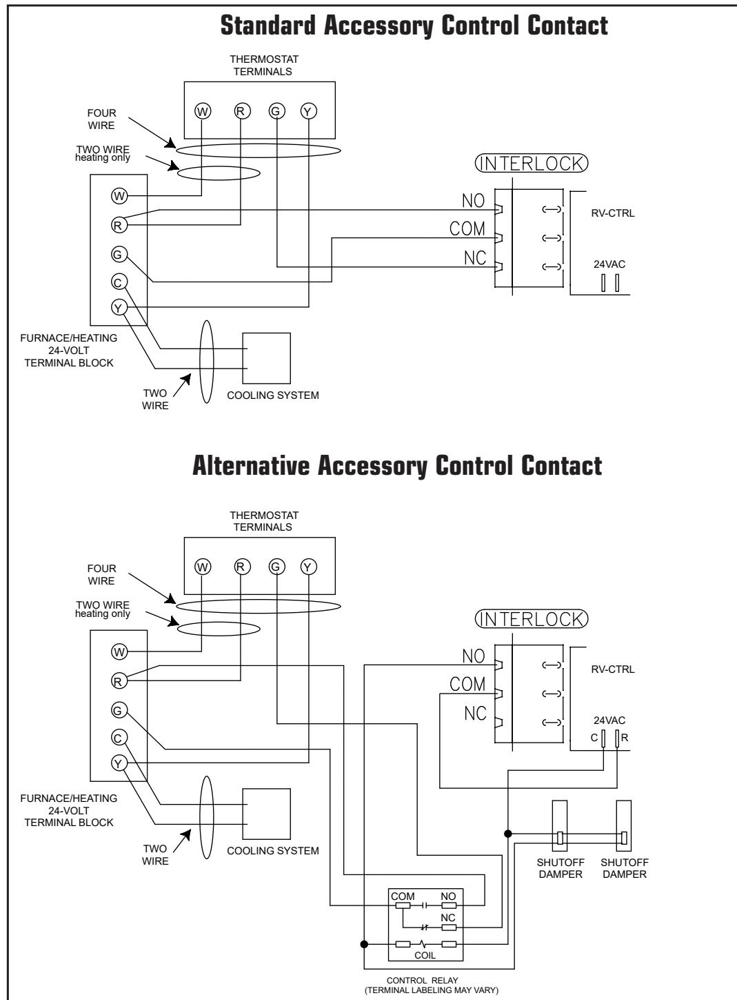
**!** **Never connect a 120 volt AC circuit to the terminals of the Accessory Control Contacts. Only use the low voltage class 2 circuit of the forced air system blower control**
