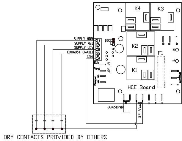
DDC CONTROL WIRING WITH DAMPER DEFROST (EXTERNAL CONTROL SIGNAL)
