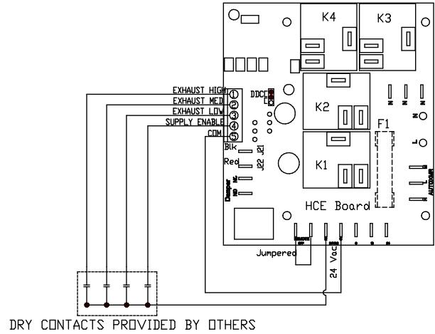
DDC CONTROL WIRING W/ O DAMPER DEFROST (EXTERNAL CONTROL SIGNAL)
