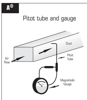
**A** The duct's airflow velocity is generally measured with a magnehelic gauge and a pitot tube.
