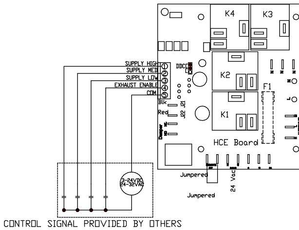
NOTE: ENSURE JUMPER ON HCE BOARD IS CHANGED FROM "NORMAL" TO "DDC"
