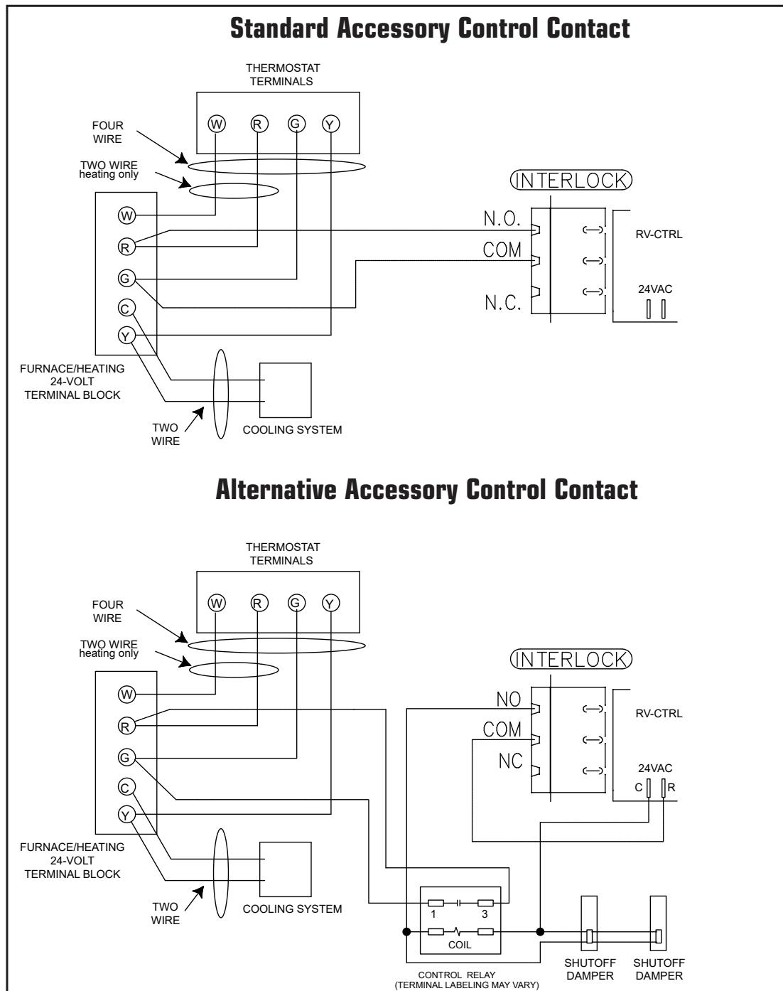
**!** **Never connect a 120 volt AC circuit to the terminals of the Accessory Control Contacts. Only use the low voltage class 2 circuit of the forced air system blower control**
