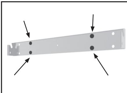
**1** Attach bracket to wall using 4 screws and washers provided.
