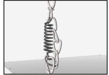
**4** Install a spring on each chain. Hook the spring in the links so a loop is created in the chain. The spring will then support the unit's weight and absorb vibrations.
