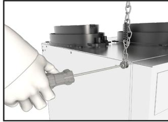
**2** Attach a hanging chain (provided) to each 19 mm (3/4") bolt (provided) in the top 4 corners of the unit and tighten.
