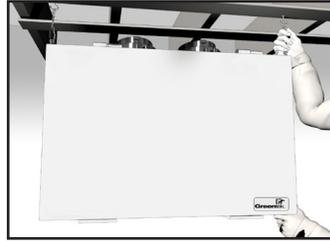
**3** Hang the unit by slipping a link onto the hanging hooks, making sure the unit is level.
