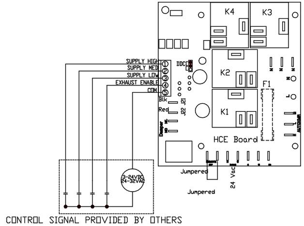
NOTE: ENSURE JUMPER ON HCE BOARD IS CHANGED FROM "NORMAL" TO "DDC"
