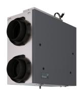
Powered by EC motors, the ENERGY STAR  $^{\circledR}$  and HVI certified PREMIER 3.0E-EC Energy Recovery Ventilator (ERV) uses a water vapor transport, durable, polymer membrane that transfers heat and moisture to the incoming air. This process helps to temper the incoming air and to maintain comfortable humidity levels.
