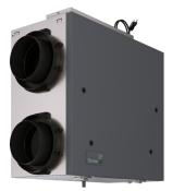
Greentek's PRS is an Energy Recovery Ventilator designed for higher static pressure applications. The unit brings a continuous supply of fresh air into a home while exhausting an equal amount of contaminated air. The energy recovery core at the center of the unit transfers heat and moisture from incoming air to the outgoing air that was cooled and dried by the building's air conditioner.
