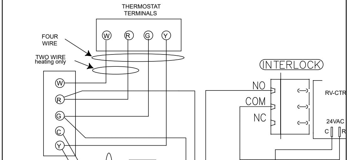
! Never connect a 120 volt AC circuit to the terminals of the Accessory Control Contacts. Only use the low voltage class 2 circuit of the forced air system blower control
