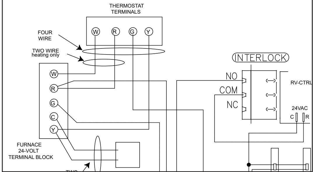
**!** Never connect a 120 volt AC circuit to the terminals of the Accessory Control Contacts. Only use the low voltage class 2 circuit of the forced air system blower control
