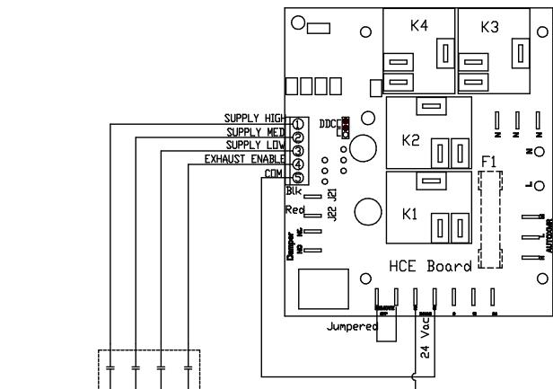
NOTE: ENSURE JUMPER ON HCE BOARD IS CHANGED FROM "NORMAL" TO "DDC"
