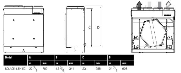
Clearance of 14" (355mm) in front of the unit is recommended for removal of core.
