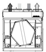
fresh air to inside fresh air from outside stale air from inside stale air to outside
