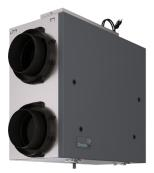
Greentek's PREMIER 2.0E is an Energy Recovery Ventilator designed for higher static pressure applications. The unit brings a continuous supply of fresh air into a home while exhausting an equal amount of contaminated air. The energy recovery core at the center of the unit transfers heat and moisture from incoming air to the outgoing air that was cooled and dried by the building's air conditioner.
