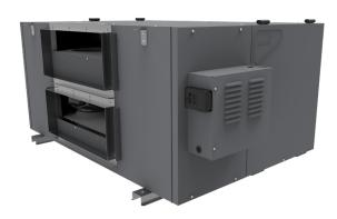
The LCH-12H Commercial Heat Recovery Ventilation system (HRV) complements today's tight buildings. Greentek Heat Recovery Ventilators (HRV) are designed to supply air into a building while exhausting an equal amount of contaminated air to the outside. The aluminium heat exchanger core transfers sensible energy between air streams resulting in tempering of the supply air and reduced loads on the HVAC system.
