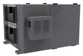
The LCH-7H Commercial Heat Recovery Ventilation system (HRV) complements today's tight buildings. Greentek Heat Recovery Ventilators (HRV) are designed to supply air into a building while exhausting an equal amount of contaminated air to the outside. The aluminium heat exchanger core transfers sensible energy between air streams resulting in tempering of the supply air and reduced loads on the HVAC system.
