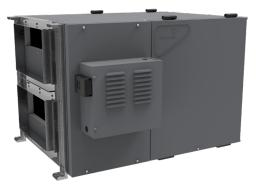
The LCH-4H Commercial Heat Recovery Ventilation system (HRV) complements today's tight buildings. Greentek Heat Recovery Ventilators (HRV) are designed to supply air into a building while exhausting an equal amount of contaminated air to the outside. The aluminium heat exchanger core transfers sensible energy between air streams resulting in tempering of the supply air and reduced loads on the HVAC system.
