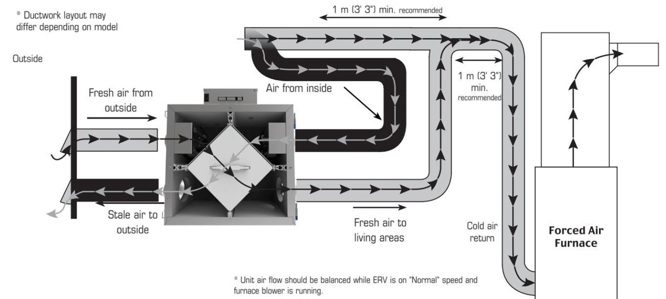
\* Unit air flow should be balanced while ERV is on "Normal" speed and furnace blower is running.
