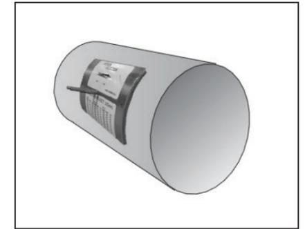
**1** Cut hole in duct and insert flow measuring station. Make sure that the flow measuring station's air direction arrow points in the direction of the airflow. Secure the flow measuring station with aluminum foil tape.
