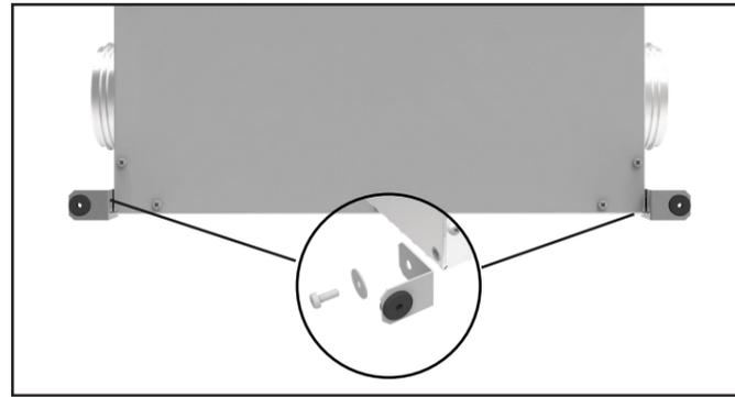
**2** Using the screw with washer mount the brackets at the bottom of the unit.
