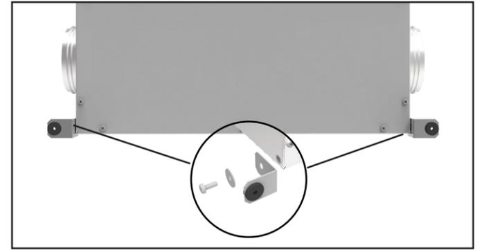
**2** Using the screw with washer mount the brackets at the bottom of the unit.
