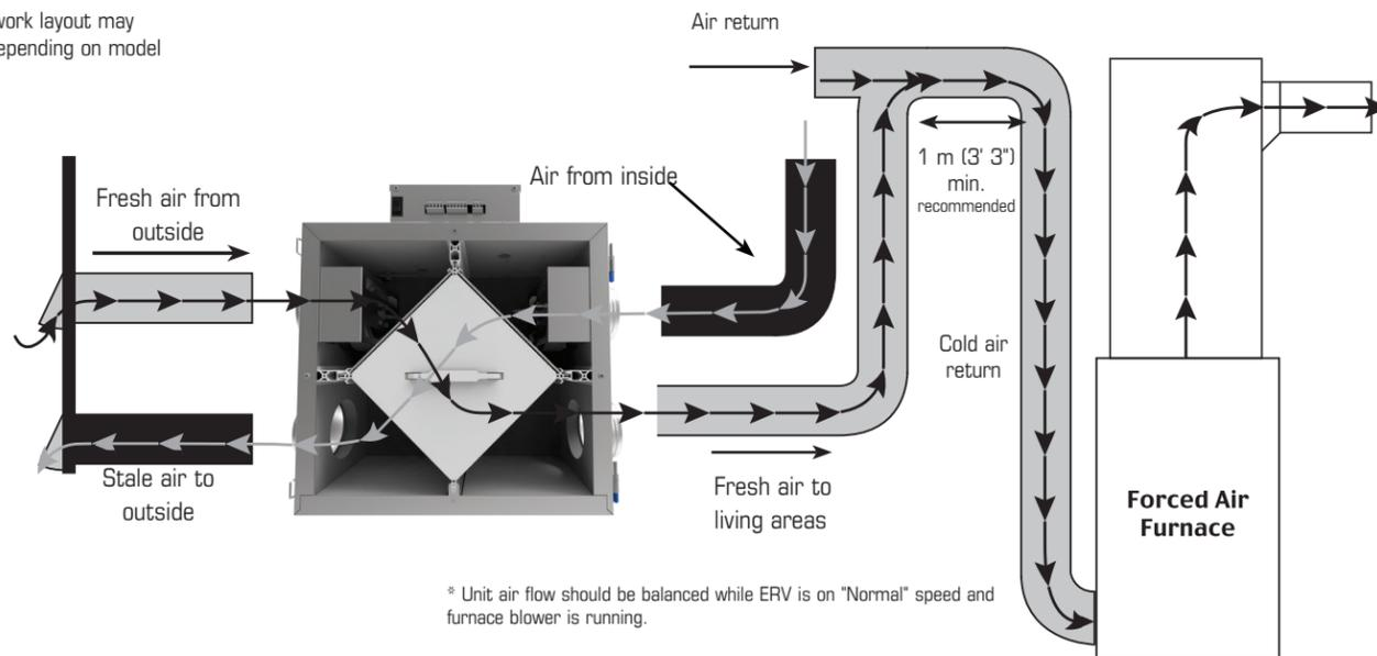
\* Unit air flow should be balanced while ERV is on "Normal" speed and furnace blower is running.
