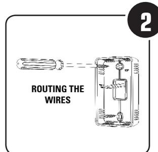
Guide the signal wires (4) through the central opening of the back plate and mount this plate to either a standard electrical device box or directly to the wall using screws. If required, use wall anchors.
