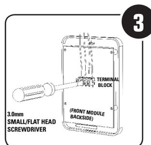
Insert the wires (4) into the terminal block, located on the backside of the front module. Secure them in place by tightening the terminal screws using a small 3.0 mm slot/flat head screwdriver (not included).
