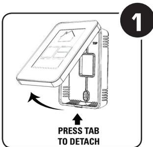
Detach front module from back plate by pressing the tab (located at the top and bottom of the control casing).
