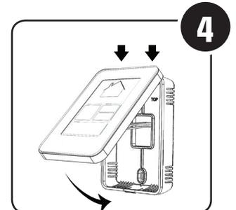
Attach front module to mounted back plate, first by hooking the top of the front module to the top clips of the back plate, then by pressing the bottom of the front module until you hear a 'click'.
