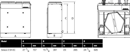
Clearance of 16" (406mm) in front of the unit is recommended for removal of core.
