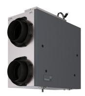
Greentek's PRS 2.0E is an Energy Recovery Ventilator designed for higher static pressure applications. The unit brings a continuous supply of fresh air into a home while exhausting an equal amount of contaminated air. The energy recovery core at the center of the unit transfers heat and moisture from incoming air to the outgoing air that was cooled and dried by the building's air conditioner.
