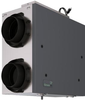
Greentek's PREMIER 1.5E is an Energy Recovery Ventilator designed for higher static pressure applications. The unit brings a continuous supply of fresh air into a home while exhausting an equal amount of contaminated air. The energy recovery core at the center of the unit transfers heat and moisture from incoming air to the outgoing air that was cooled and dried by the building's air conditioner.
